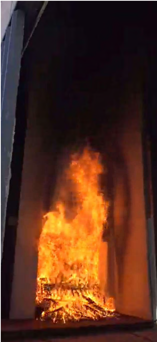
FIGURE 17: CRIB COLLAPSE AND 30 MINUTES
