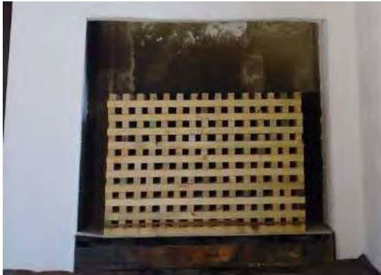
TIMBER CRIB INSTALALTION
